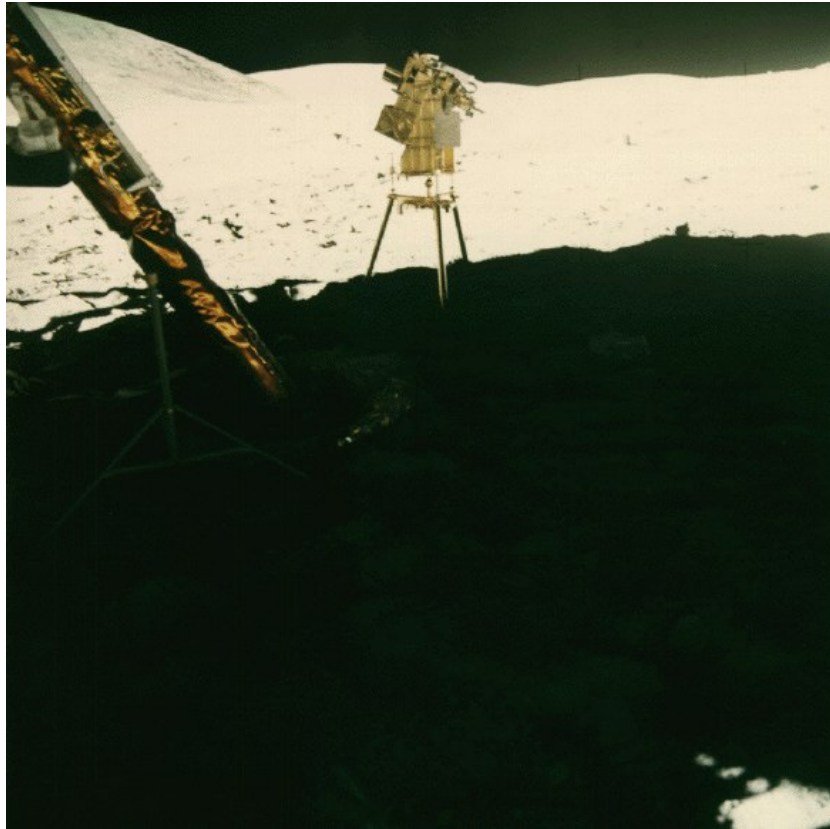
Apollo 16 Far Ultraviolet Camera/Spectrograph in the lunar module shadow in 1972. This photograph shows the instrument, not one of its ultraviolet star fields. Credit: NASA/Apollo 16. Resized.
